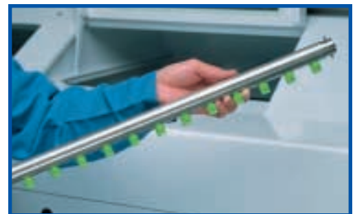
FIGURE 1: Removable spray bar and nozzle assembly.
