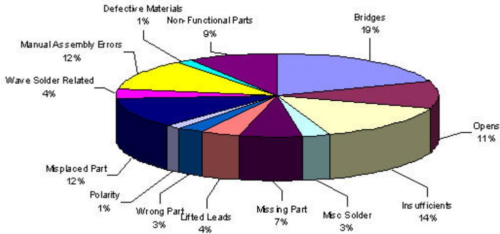
Figure 1 - Defect Chart for All Electronics Assemblies
