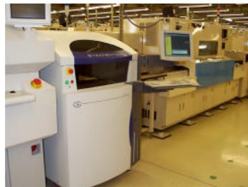
**Figure 6 - The 100-Percent Solder Paste Inspection Machine Installed In-Line at SMT Facility**
